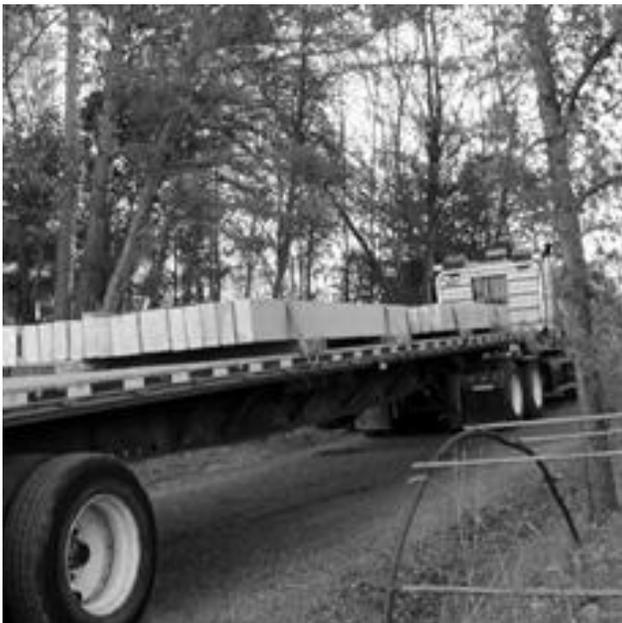
The Lake Shamineau Association has partnered with Scandia Valley Township to install horizontal concrete planks at the public access at the east end of the lake. The planks will provide a firm base for vehicles and trailers launching boats. It is hoped that this will stop the bottom erosion that takes place when boat owners need to rev their engines to make it onto their trailer.
