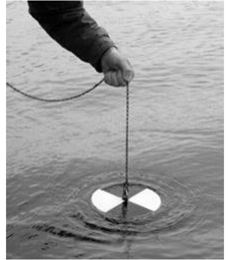
A Secchi disk is lowered and raised to find the depth of water clarity. This reading is one of the factors in the formula to determine Trophic State Index.
